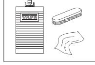
After each use, clean the pipe stopper with a solution of water and detergent. Never use solvents, hydrocarbons and other aggressive cleaning agents.
